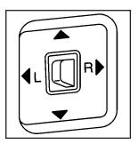
Vehicles with outside power mirrors have controls on the driver's door armrest.
